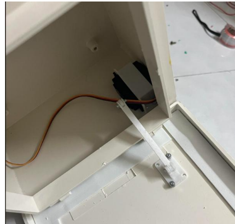
Figure 6 cabinet with 3D-printed hinge and servo (interior)
