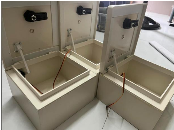
Figure 5 Cabinet with 3D-printed hinge and servo (exterior)
